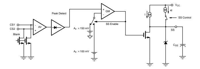
Figure 7. Current-Sense and Soft-Start Circuit Block Diagram
