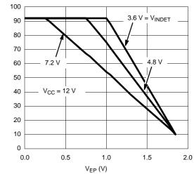
Duty Cycle vs. V<sub>INDET</sub> @ 25°C V<sub>EP</sub> = 1.2 V, V<sub>CC</sub> = 9.5 V
