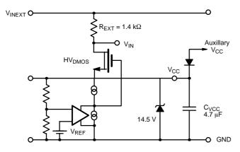
Figure 6. High-Voltage Pre-Regulator Circuit
